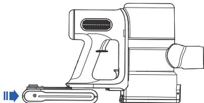
**Removal:** press the battery release button and pull it out for removal.
