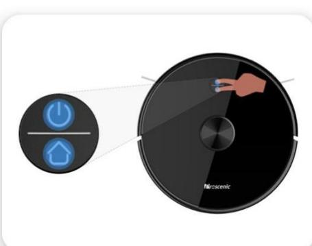
1. Hold "P" and "H" buttons for 5 seconds with two fingers, the machine will have a prompt sound for pairing network
