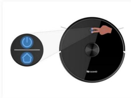
1. Hold "O" and "H" buttons for 5 seconds with two fingers, the machine will have a prompt sound for pairing network
