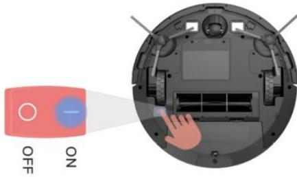
1. Please check whether the robot is turned on and the indicator light is on
