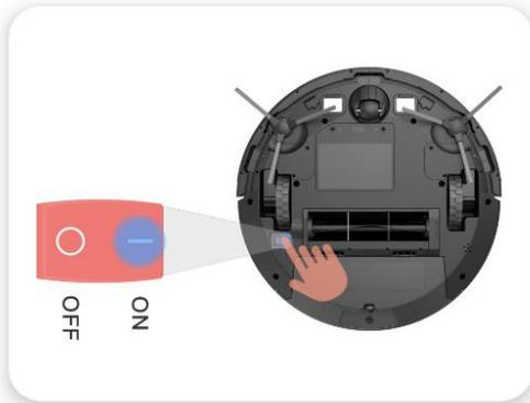
1. Please check whether the robot is turned on and the indicator light is on
