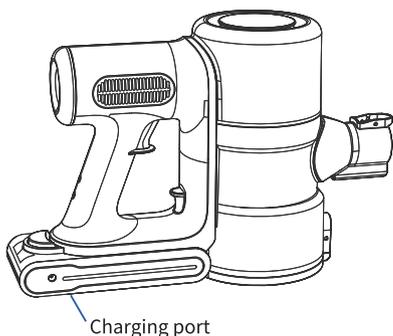
2. As shown in the picture, after the battery is removed, insert the charging plug into the charging port on the battery, the indicator light is flashing blue, indicating that it is charging; the indicator light is solid, indicating full charge.
